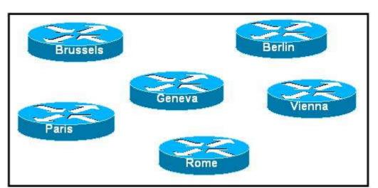
Refer to the exhibit. All of the locations are going to be connected by a new WAN solution. If Frame Relay is selected as the solution, how many physical circuits are required to create a Frame mesh topology?
