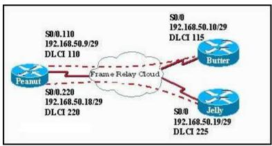
Refer to the exhibit. A ping is sent to address 192.168.50.10 from the Peanut router. Which DLCI will be used to send the ping?
