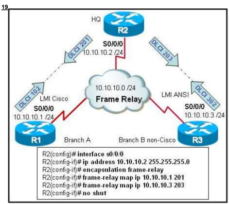
Refer to the exhibit. Router R2 is part of a Frame Relay network that uses OSPF for IP routing. After the commands that are shown are entered, R2 will not exchange OSPF information correctly. What is the likely cause?
